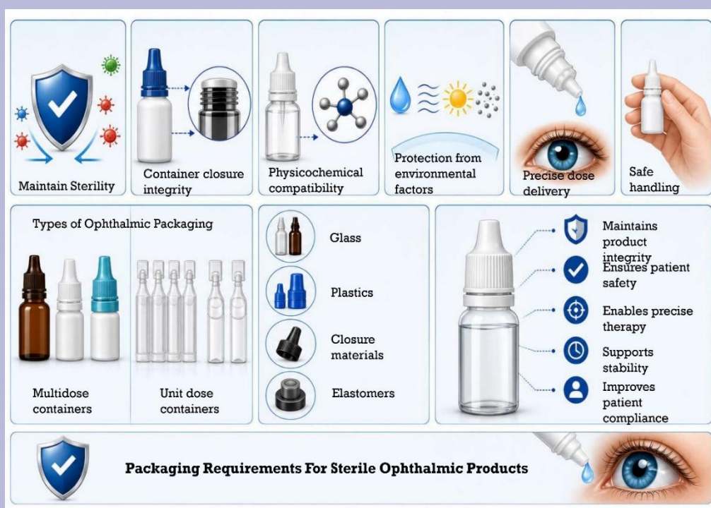
Figure 2. Schematic representation of packaging requirements for sterile ophthalmic products
